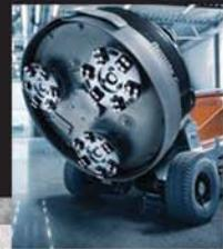
Redi-Lock diamond tools are perfect for concrete grinding applications, such as aggregate exposure, preparation for tiling floors, removal of epoxy coatings and sealers as well as flattening.
