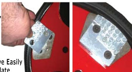
**B** are rotating Planetary heads, for flattening & fine finish. Tools are attached with velcro, using special double-sided pucks which allow for easy change of tools.
