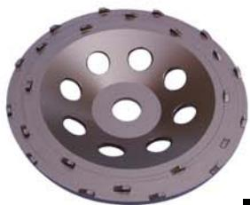
Poly Crystalline Diamonds make for extremely aggressive removal of glue, epoxy, mastics & the worst of the worst coatings. The hardest substance known to man stays sharper longer under extreme conditions. Use dry. 5/8"-7/8" bore.
