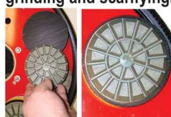
Attach Easily - Velcro & Direct Attach To Rotating Heads.
